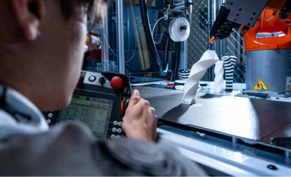
■ Student Jason Pieck works with a multi-axis 3D printer, which is capable of producing parts in a variety of complex shapes.
