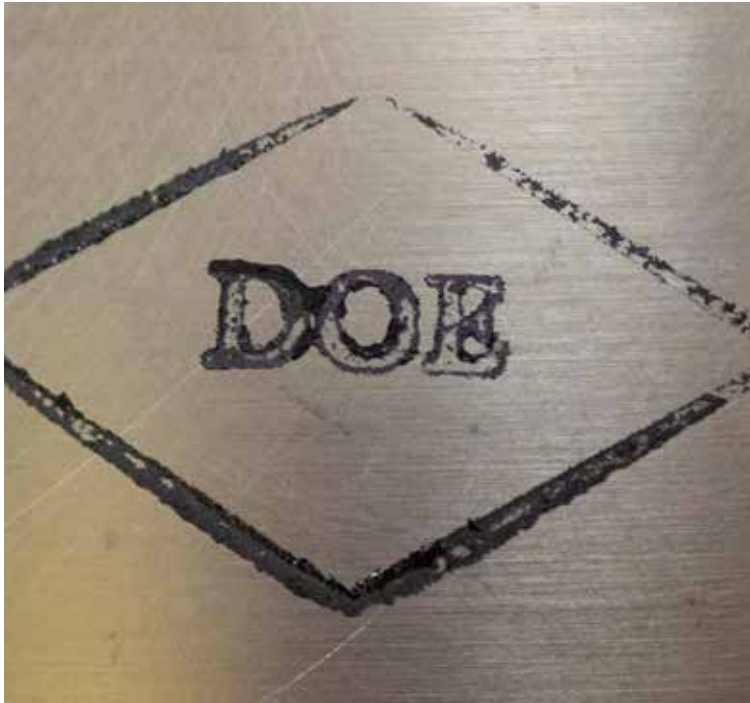
■ A diamond stamp indicates that a component has met or exceeded all quality and design requirements established by its design agency, which in the case of the W87-1 pit is Lawrence Livermore National Laboratory.
