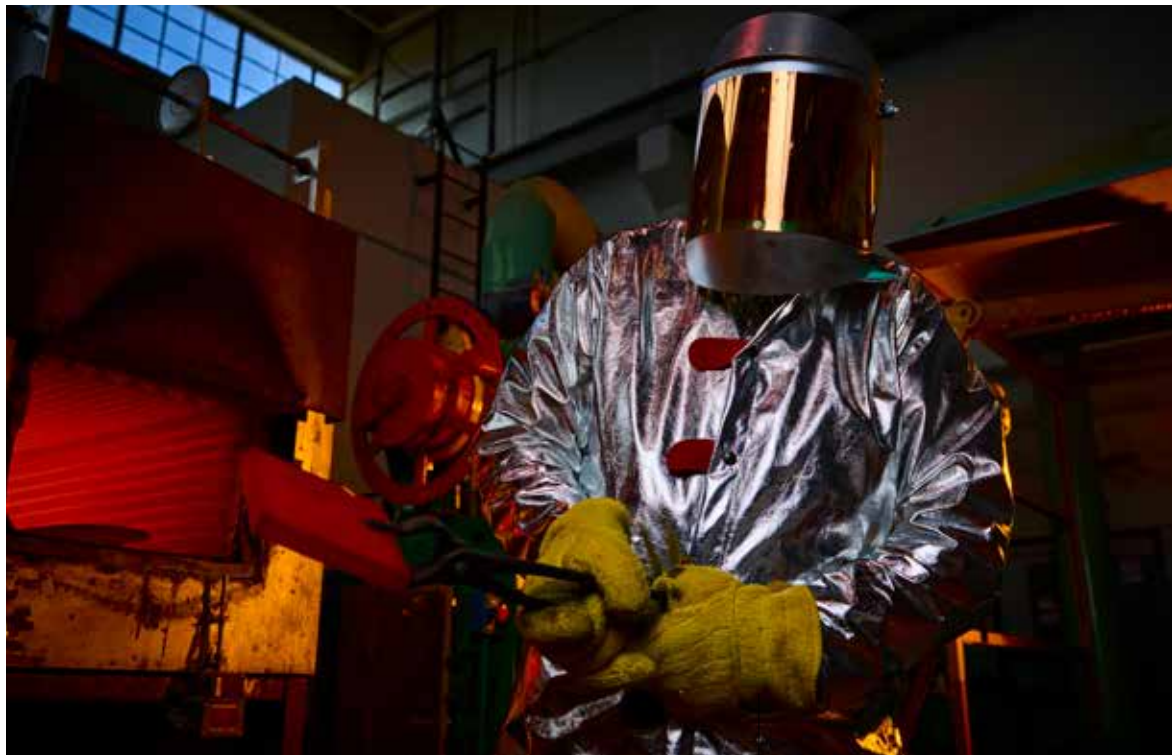
■ A deformation processing technician removes a hot billet of uranium from the pre-heat furnace.
