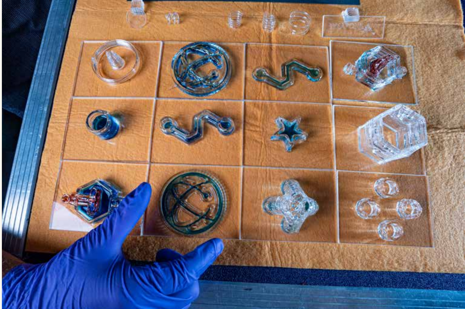
■ Glass additive manufacturing is still in the early stages of development, but the technique might one day be used to produce hard-to-make glassware.
