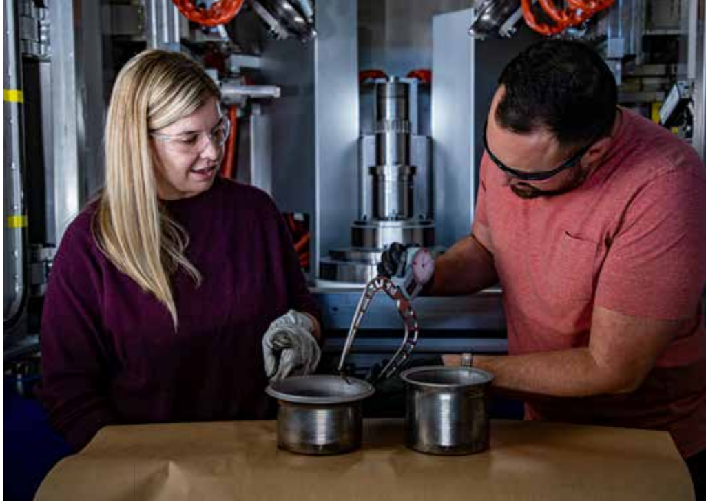
■ Engineer Kayla Molnar and scientist Matthew Zappulla take measurements and examine steel cups made on Sigma’s metal spinning machine.
