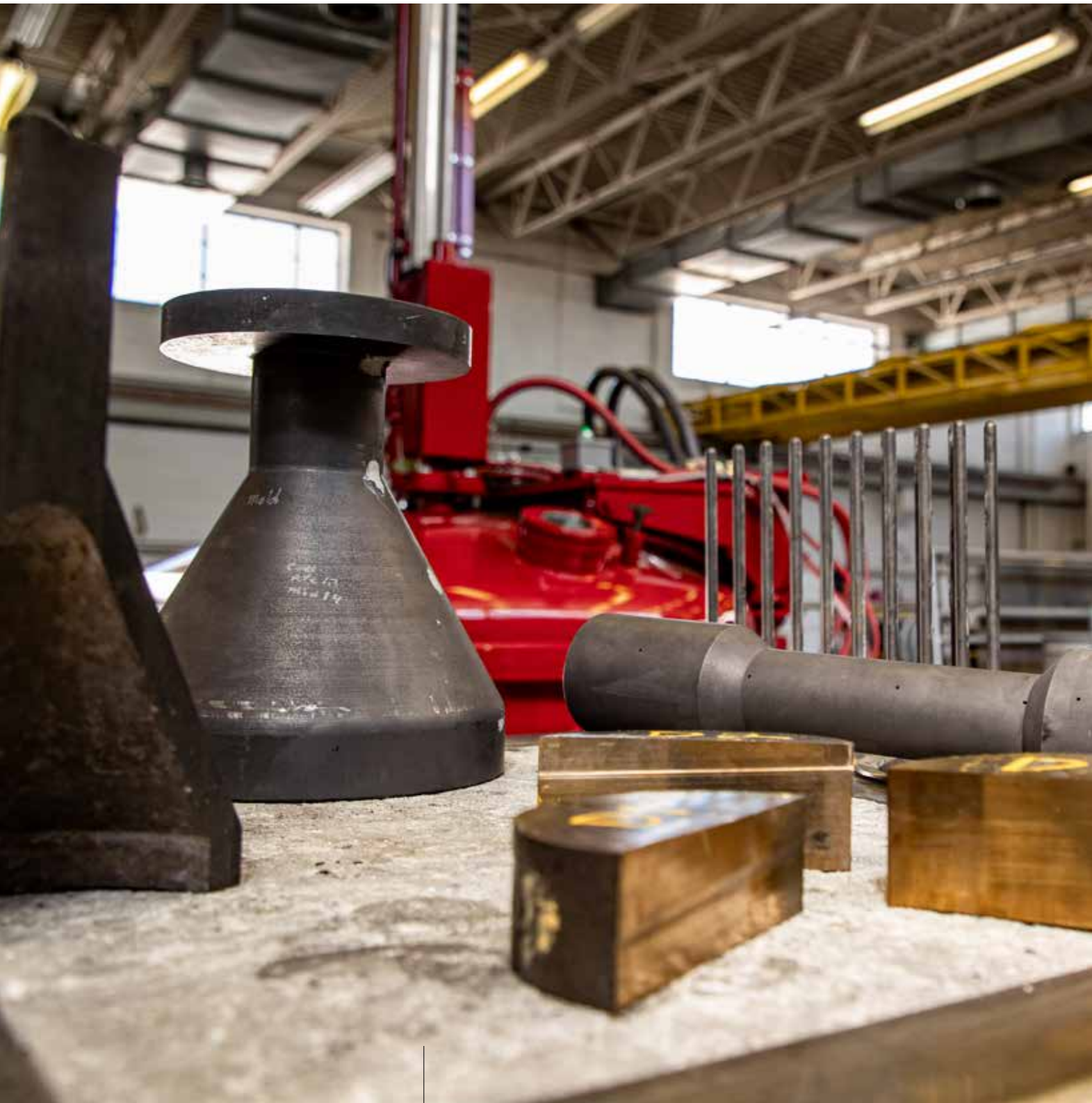
■ Inside Sigma's foundry are a gantry crane (yellow), an induction furnace (red), and an assortment of graphite and uranium parts (foreground).
