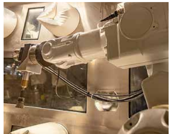
■ APPA works inside a glovebox.
