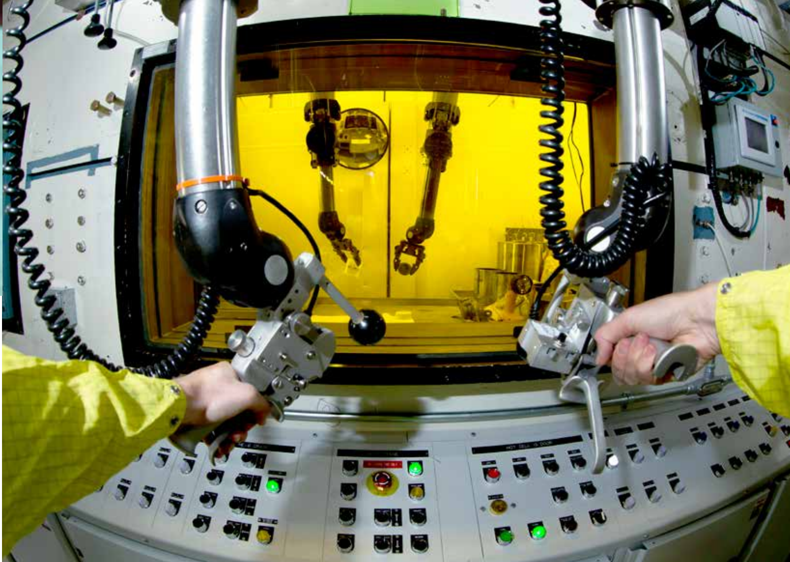
■ Inside a shielded chamber, robotic arms are used to handle radioactive medical isotopes.
